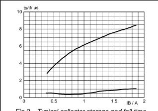
Fig.9. Typical collector storage and fall time.  $ts = f(I_B)$ ;  $tf = f(I_B)$ ;  $I_C = 4.0 \text{ A}$ ;  $T_j = 85 ^{\circ}\text{C}$ ; f = 16 kHz
